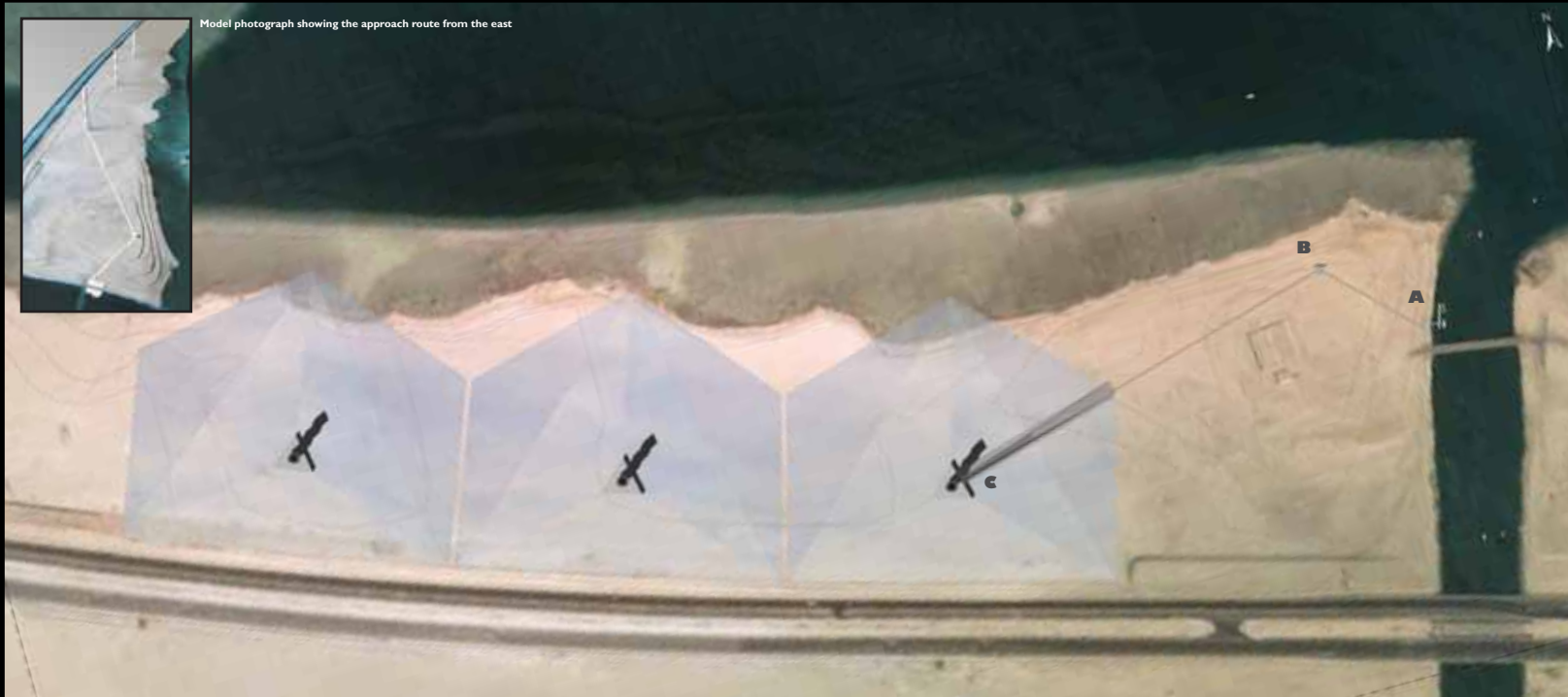
Plan view of the three solar collectors and the pedestrian approach route from the east: A is the boat jetty, adjacent to the bridge; B is the viewing pavilion at the high point of the site; C is the base of the publicly accessible Light Tower
