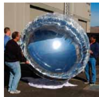
Cool Earth: inflatable solar module
