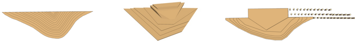
Figure 4: Induced Meander "Deflectors" (plan view)
