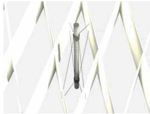
DETAIL 3 - LED LIGHT ATTACHMENT TO PLASTIC STRUCTURE
